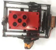
Six-rotor VESPA drone with RedEdge multi-spectrum payload
