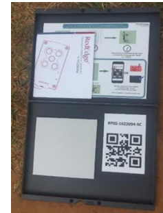
Ground control point panel and calibrate equipment to ensure consistent data collection for processing
