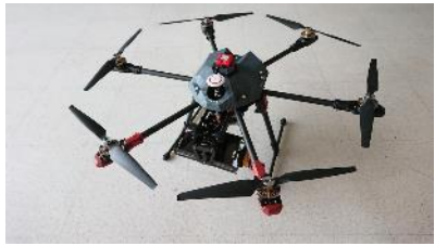
Six-rotor VESPA drone with RedEdge multi-spectrum payload
