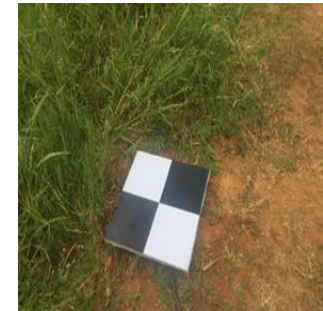
Ground control point panel and calibrate equipment to ensure consistent data collection for processing
